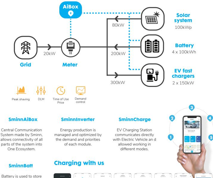
Battery is used to store the energy from the sun and grid load. The system will make sure to charge in the lowest rate possible.
